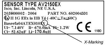
Figure 2-20 AV2150EX Sensor Cable Labels
